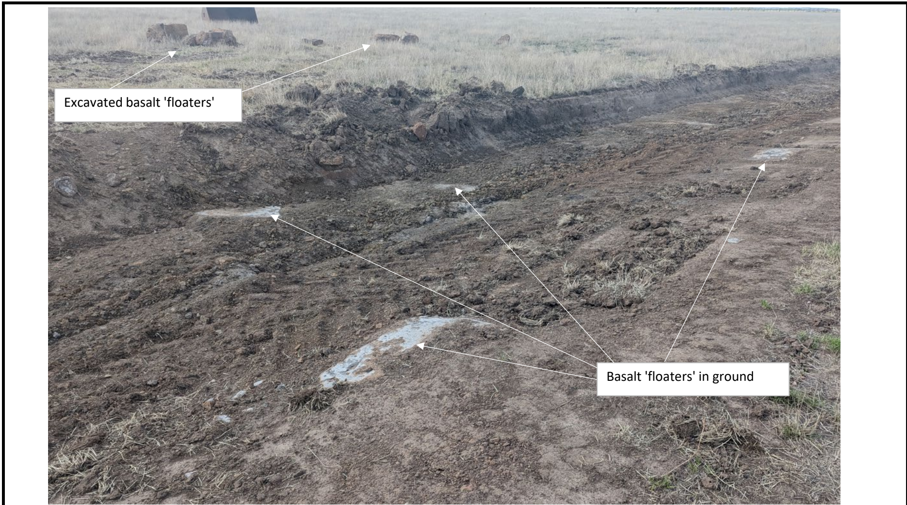
Example of basalt 'floaters' in residual clayey soil matrix exposed in drainage works occurring on a farm, close to proposed location of WTG T40. Excavated boulders were predominantly tabular, very high strength, and up to 1.5 m long.
