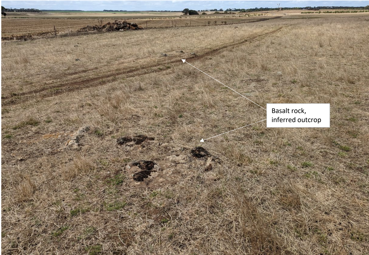
Basalt outcrop at surface at location of proposed WTG T80. This was not widely encountered during the site visit. Could potentially be corestones (or 'floaters') in a soil matrix.
