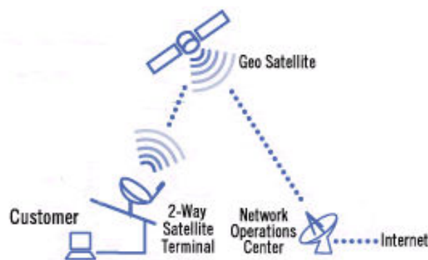
Figure 1 Two-way connection to the internet via satellite [1]
