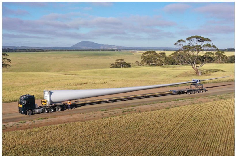
Figure 6.7 Example wind turbine blade being transported (Source: ABC News, 2020)
